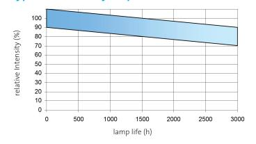
The typical **lamp life is approx. 3.000 hours** (guaranteed lamp life 2.000 hours). It is possible to readjust the lamp output in order to maintain the intensity.
